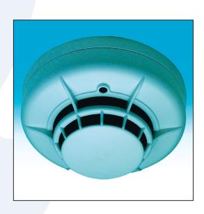
The HRZ-1002 detector also has an integral LED, which illuminates to provide a local alarm signal. This latches on, and remains illuminated until the detector is reset by a momentary power interruption. An optional remote LED annunciator may be used to repeat any alarm signal.
