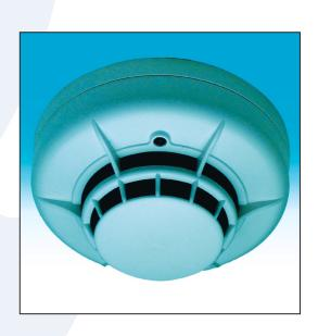
The HRZ-1005 detector also has an integral LED, which illuminates to provide a local alarm signal. This latches on, and remains illuminated until the detector is reset by a momentary power interruption. An optional remote LED annunciator may be used to repeat any alarm signal.
