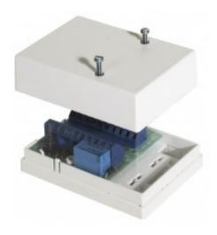
The RC 020 is a relay card with two relays and dual (2x) alternating (NC/NO) functions. Connection is provided via screw terminal with wire protection. Active relays are indicated by LED. The card also has an antitamper switch to protect against unauthorised opening if the card is installed, for example, in a JB 200 box.
