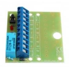
The RC 010 is a relay card with a dual (2x) alternating (NC / NO) function. Connection is provided via screw terminal with wire protection. Active relay is indicated by LED. The card also has an anti-tamper switch to protect against unauthorised opening if the card is installed, for example, in a JB 200 box.
