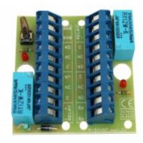
The RC 020 is a relay card with two relays and dual (2x) alternating (NC/NO) functions. Connection is provided via screw terminal with wire protection. Active relays are indicated by LED. The card also has an antitamper switch to protect against unauthorised opening if the card is installed, for example, in a JB 200 box.
